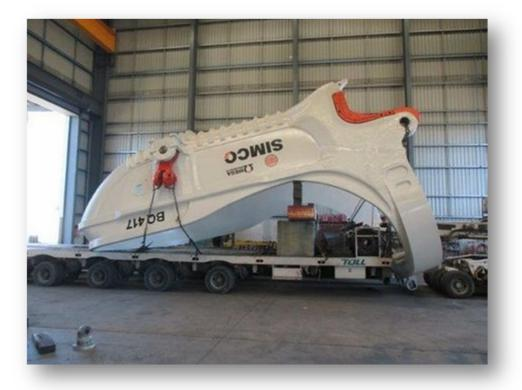
The giant dragline bucket loaded onto the truck prior to being taken from the workshop to Blackwater. Photo Alan Quinney
