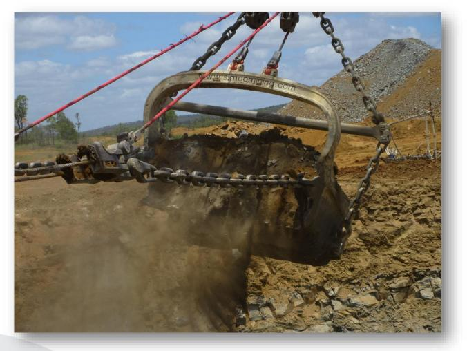
The design of the Bucket features low sidewalls compared to conventional Buckets for weight reduction and material flow assistance.
